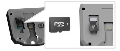
Insert card: Power off the device, open the cover on the backside of the monitor and insert the TF card according to this chart.
