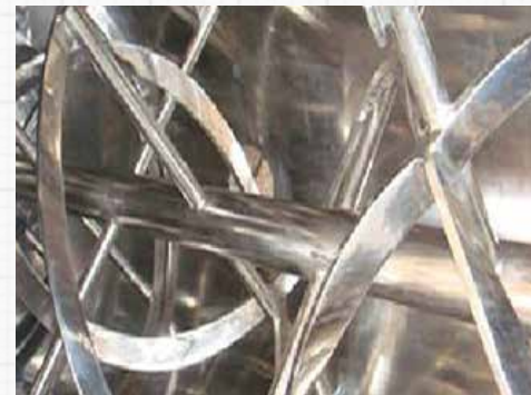
Double ribbon design from inside of Ribbon Blender
