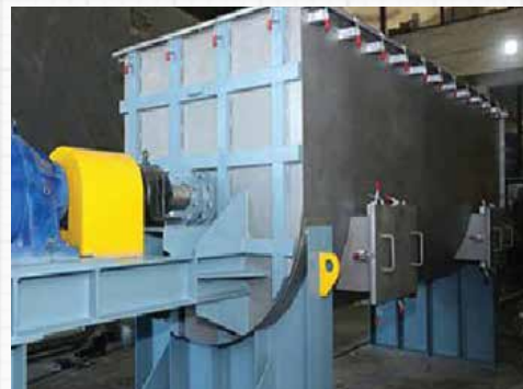
Hellical Gear Drive arrangement based Blenders
