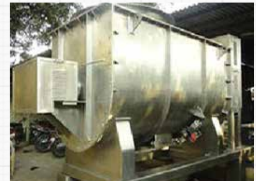
Ship gear and Pinion type gear mechanism based Blender
