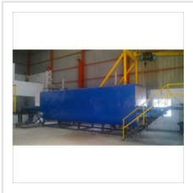
Bitumen Drum Decanter Plant (Chain)
