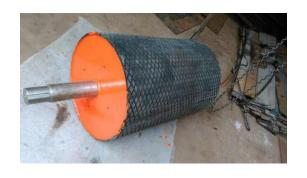
Magnets and An-Isotropic Hard ferrite Magnets and operate without the need for power supplies. The magnet system is available in tow types: with Longitudinal polar field disteibution for use with low levels of iron contamination and thin material layers, and with lateral polar field distribution for greater material thickness and larger iron particles.
