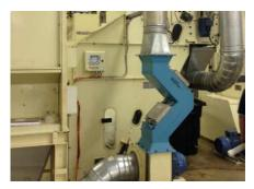
Made from high coercively permanent magnets. Very powerful magnetic plates hinged on sturdy, S. S. Housing arrest all the ferrous particles from the material and prevent damage to the machinery. The plates can be easily swung open and cleaned.
