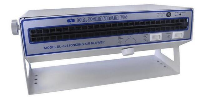
Great amount of wind, width scope ion annihilator The neutral time is quick, the ion wind cover area is big, has the heating function, is suitable specially for professions and so on printing, electron, plastic. The amount of wind may adjust in the 70-120CFM scope, ionic equilibrium voltage for 0V±10V.
