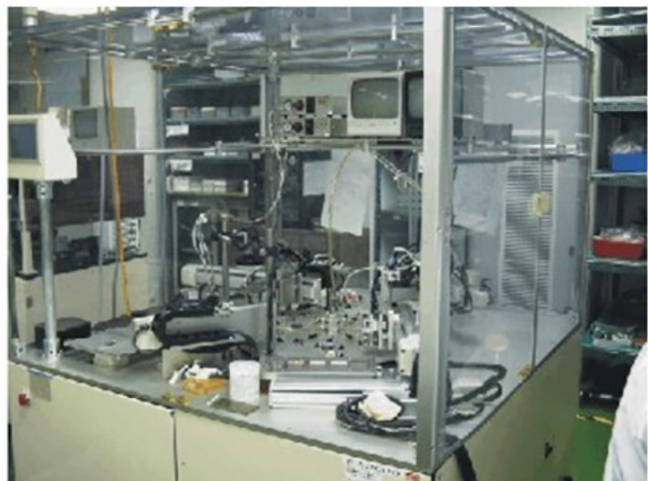
BLANK MOUNTING - Prepared crystal blanks are mounted onto substrates for surface-mount products
