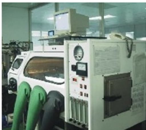
RESISTANCE-WELDER - Resistance weld chamber. Crystals and oscillators are sealed under a controlled atmosphere; units are 'back-filled' with nitrogen during the hermetic sealing process
