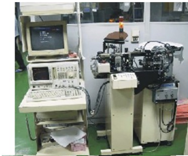
PACKAGE ASSEMBLY - Automatic tacking of package lids prior to seam welding surface-mount products
