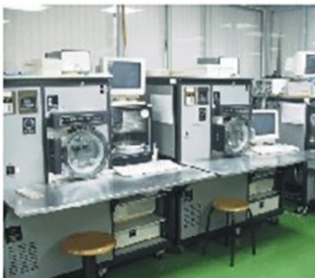
FINAL ADJUST - Oscillator final adjustment equipment. Crystal units are adjusted to final frequency under computer control.
