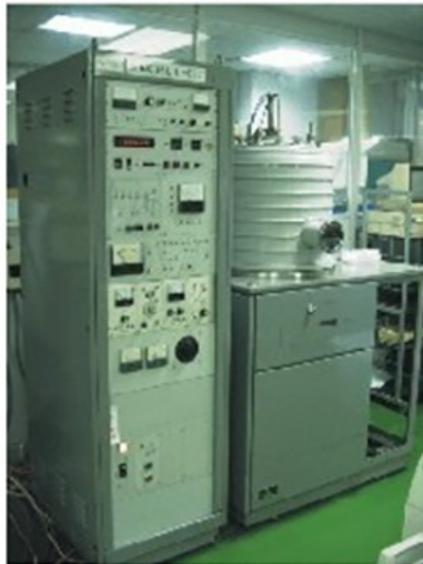
PLATING UNIT - a vacuum/heat process, used to plate silver or gold electrodes onto crystal blanks
