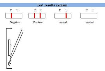
To develop color on C line only: negative; To develop color on both C line and T line: positive; To develop color on T line only: invalid; Not to develop color on both C line and T line: invalid.
