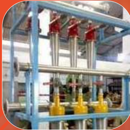
Germ Separation Cyclone
