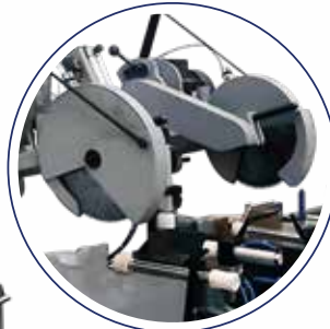
Minimum Distance between the Head is 350MM
