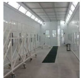
Industrial Paint Drying Oven
