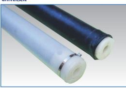
Universal-Make Tube diffuser is an assembly of high-quality EPDM/SILICON membrane of 63mm diameter and 610mm length on standard PVC pipe and tightly held by SS 304 clamps to ensure trouble free operation. The air inlet is through rigid PVC Hub designed to provide uniform air distribution throughout the tube. The minute pores on the membrane behave as NRV to prevent water from entering the tube. 63X610mm comes with 3/4" SS adaptor for easy mounting of diffusers to the diffuser skid.
