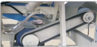
POWER TRANSMISSION DRIVE SYSTEM WITH GEAR BOX
