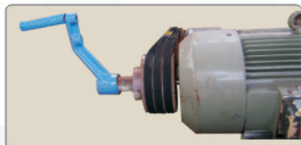
EMERGENCY HAND LEVER TO ROTATE DRUM
