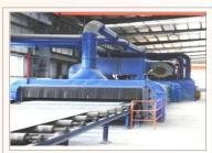
This type of system provides complete surface treatment for plates. A typical plate preservation line consists of ---Inlet Roller Conveyor -----Pre Heater-----Shot Blasting machine -----Automatic Spray Painting Line -----Slat Conveyor------Baking or Drying Oven------Outlet Conveyor.
