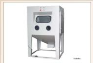
Suction Blaster works on induction-suction principle of abrasive delivery. The suction machine, also known as a siphon, is most commonly used for light production and general-purpose cleanup. In this type of unit, air passes through the gun, creating a siphon action that sucks up abrasive and delivers it to the nozzle where it is propelled out to the target.
