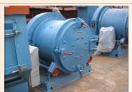
These types of machines are widely used in small or medium size iron, steel, alloy and non-ferrous castings, forgings, heat treated parts, pressings and fabrications at the lowest possible cost. It is ideal to use in applications requiring the blasting of small, flat, and light components.
