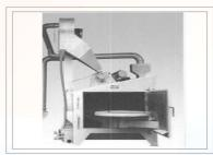
Table type shot blast machines are designed and built as fully integrated blast cleaning systems to handle larger and/or more fragile castings than barrel /tumble machines. Machine consists of door with a work table for handling job/component. Rotational mechanism of table ensures that the upper portion of the component under process will get exposed to the blast stream for through cleaning.
