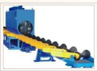
These types of machines are best suitable for blasting round objects which includes, Pipes, Tubes, solid Bars, Shafts etc. It consists of Diabola Type/Skew Type Material handling system, which helps the components to move forward along with rotational movement. Both movement ensure that the component under process experience the complete blast stream exposure.
