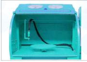
This accessory is opted, so that operator can rotate the job inside the blast cabinet to blast the other side of the components. This save the time of getting out the component and again placing them with other face in front position.
