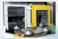
Indexing table type SPM are used to cater the gears and shafts of the different industries, for inducing a residual compressive stress in its surface thereby improving its resistance to fatigue failure.
