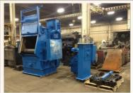
These machines are basically designed for batch type operation. This type of machine consist of a tumble cupped shaped rubber belt work conveyor. Tumbling action of the rubber belt conveyor ensures that each and every portion of the component which is under process, will get exposed to the blast stream for through cleaning.
