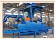
In stone and marble industry shot blasting process is used for preparing roughness on the outer surface of components, so that bounding with the cement or any holding chemical remain sturdy & also, to make them non-slippery.
