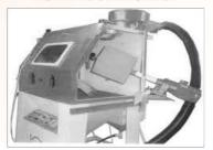
This accessory is generally used for catering the small jobs, so that they can be blasted in a one lot. Continuous tumbling action ensures complete exposure of blast stream. Thus batch production is possible with this accessory.
