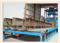
The roller conveyor shot blasting machine is best suitable for the shot blasting of round/square/hex bars/rods/plates/ H or I beams/channels/angles/flats/strips/structural sections and supports etc.
