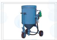
Portable Abrasive Blaster is mostly used sand/shot blasting machine in industry because of its easy to handle technique and easy portability. This blaster is equipped with wheels, so that it can be taken from place to another without any hustle.
