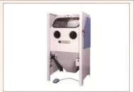
Wet blasting, also known as slurry blasting is similar to a dry blasting. However, unlike dry blasting, wet blasting uses a third element – liquid – to enhance the levels of surface finish that can be achieved. It works as well removing oily scale and corrosion from engines as it does etching aviation composites or adding precision textured finishes to delicate medical instruments.
