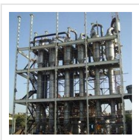
Multiple Effect Evaporator Plant For
