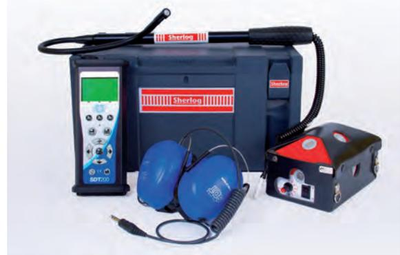
The Sherlog "MATE" kit includes the **SDT200** receiver which is a high quality ultrasonic receiver which allows to easily identify areas where compression is affected and evaluate measurements which are shown digitally on the LCD display.
