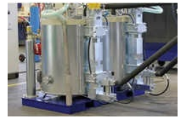
Epoxy Resin Mixing And Pouring Plant
