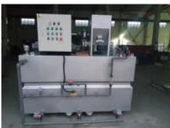
Three Phase Automatic Dosing Unit
