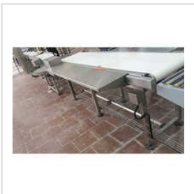
Food Processing Conveyor
