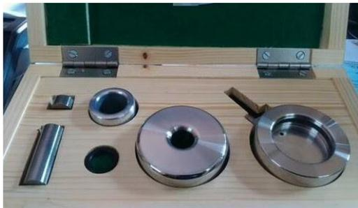
We regularly manufacture dies made from Hardened Alloy Steel for all Powder Compaction Applications. These Dies are used to form circular pellets for IR/ FTIR / XRF Solid Sampling. Dies made from Hardened Alloy Steel achieve a high hardness & hence take high pressure. Also, this material is corrosion resistant. Each die consists of two piece outer die body, punches (anvils), pusher rod & pellet removal ring. carbide have to be handled with extreme care.
