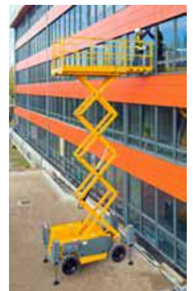
GB 139 Self Propelled Scissor Lift Cap: 200 to 500 kgs Lifting ht: 6 to 10 Mtr
