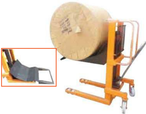
GB 123 Paper Reel Stacker Cap: 500/1000 kgs Max ht: 500/1000/1500 mm
