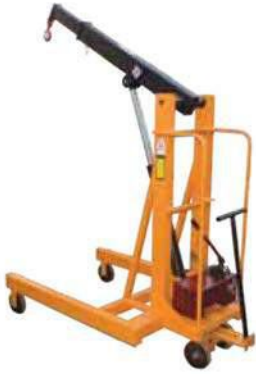
GB 141 Manual Mobile Floor Crane Cap: 500 kgs to 5000 kgs Max hook ht: 3100 to 5000 mm Min hook ht: 500 mm
