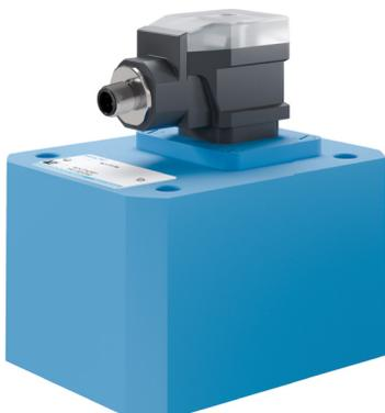
VC flow meters with IO-Link technology are based on standard VCs with one or two sensors. Unlike standard or encoder versions which always send a square-wave signal to the electronics, IO-Link devices have the added capability of internally computing concrete measurement values. Therefore, these flow meters lend themselves for use in classic PLC and in IO-Link infrastructures.
