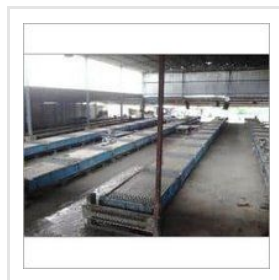
Precast Prestressed Concrete Wall Mould
