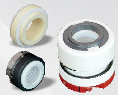
Seal Type 74 Mechanical Seal are Externally Mounted Reverse Balanced Design Seal having 'O' Ring as a Secondary Sealing member. Secondary Sealing member can be changed as per Chemical Compatibility. All metal components including springs are Isolated from the Sealed, Aggressive Medium. Simple checkout method function and cleaning possibility as this Mechanical Seal located easily access outside the pump. Especially design Clamp Ring eliminate Slipping on Shaft..
