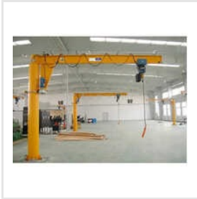
Pillar Mounted Jib Crane
