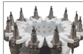
Rotary Type 12-positions Auto Tool Changer Reducing Time
