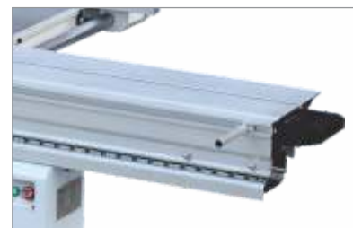
European type sliding with multiple locking point
