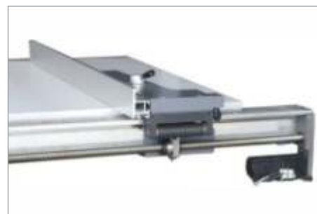
Gauge Automatic Lifting by servo motor which makes the cutting more accurate
