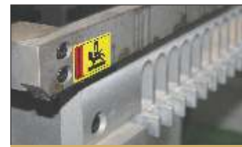
Pressure Clamp with sensor prevent accident
