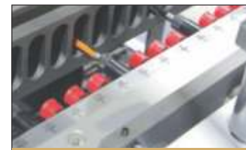
While horizontal high speed drill insure high accuracy in Ply & solid wood
