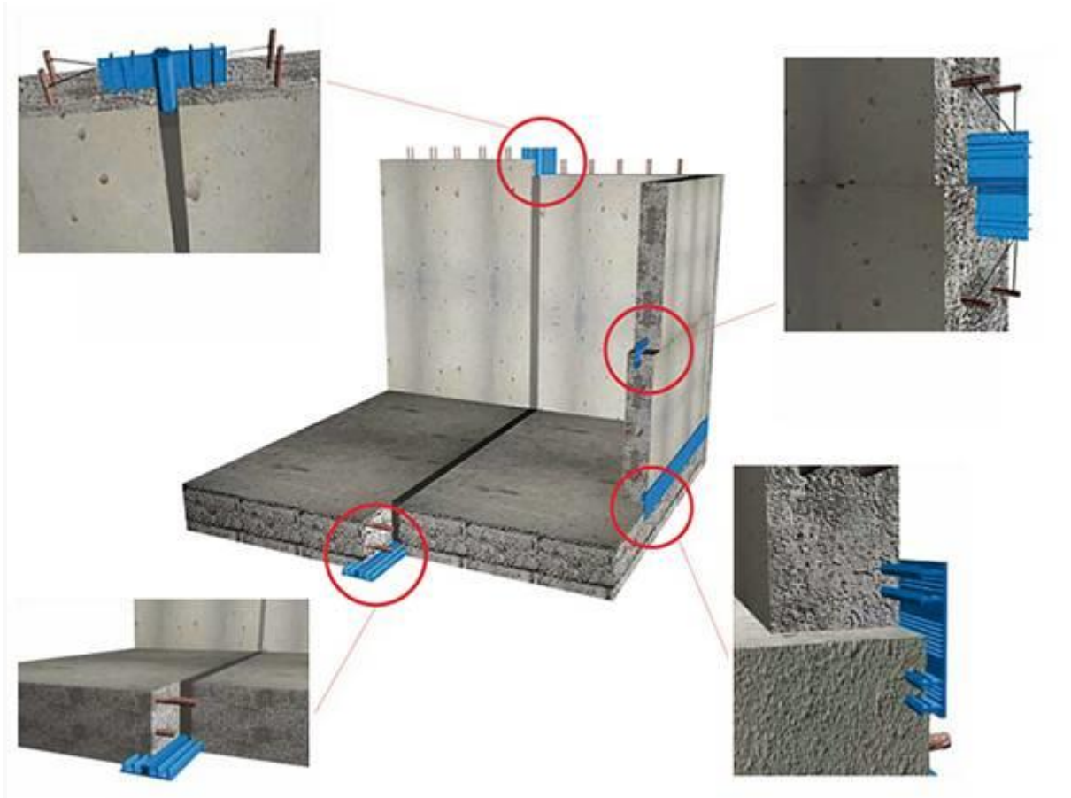
External & internal waterstop concrete pouring
