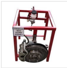
Working Model Of Disk Brake With Caliper
