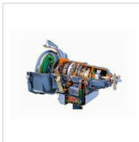
Cut Section Automatic Transmission Gear Box
