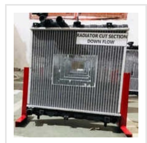
Model Of Radiator Cut Section Down Flow
