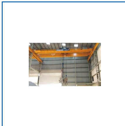
DOUBLE GIRDER EOT CRANE
