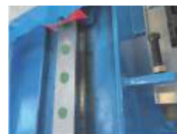
Roller linear guides for greater loads
