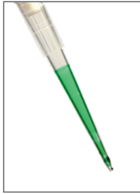
Conventional tip after dispensing 100 µL sample.
