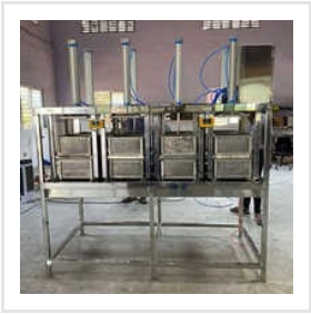
200Kg Automatic Paneer Press Machine
