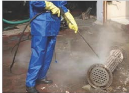
Tube Bundle Cleaning - External
