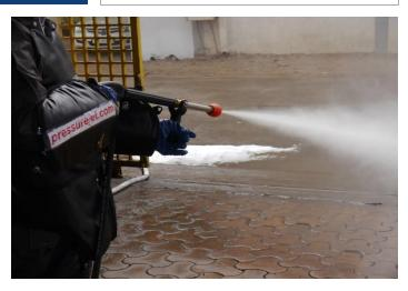
PressureJet / AAAG, India's leading fire fighting accessories manufacturers introduce complete Ultra High Pressure (UHP) fire suppression systems. This system consists of PressureJet™ UHP reciprocating plunger pumps and high quality accessories. UHP fire pump with forged alloy steel crack shaft and forged connecting rod are the UHP of ultra high pressure fire pump which offers highest reliability across all Indian manufacturers.
