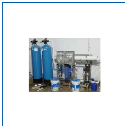
INDUSTRIAL RO SYSTEM
