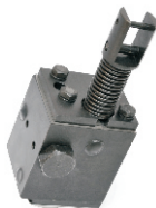
Sr No.: 5025-A : HYD. LIFT DISTRIBUTOR ASSLY. SWARAJ [O/M. 2 PIN] Ref. No.:
