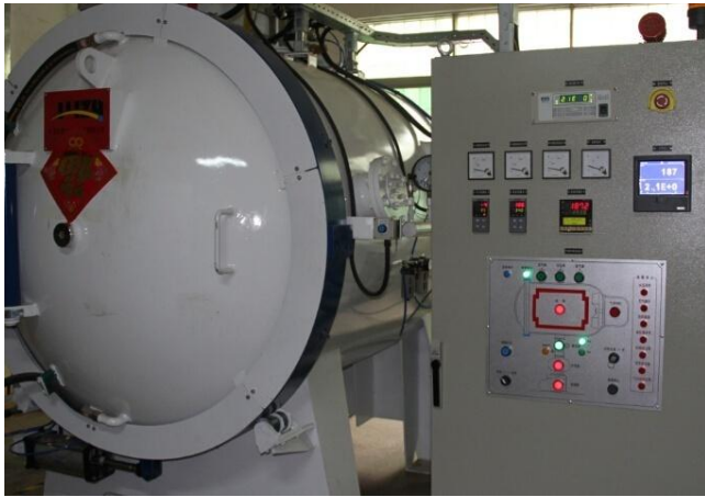
Vacuum heat treatment oven
