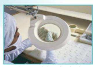
Needle inspection under illuminated magnifying glass Checking minute defects
