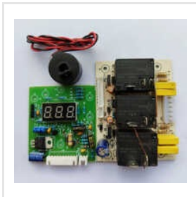
AC Stabilizer Circuit With Relay Display
