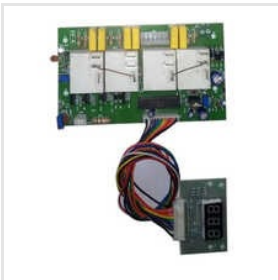
Structure Stabilizer Circuit Control Card
