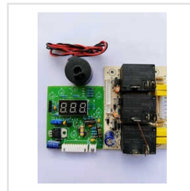
Automatic Voltage Regulator (AVR)
