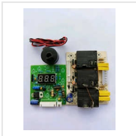
Voltage Regulator Control Card
