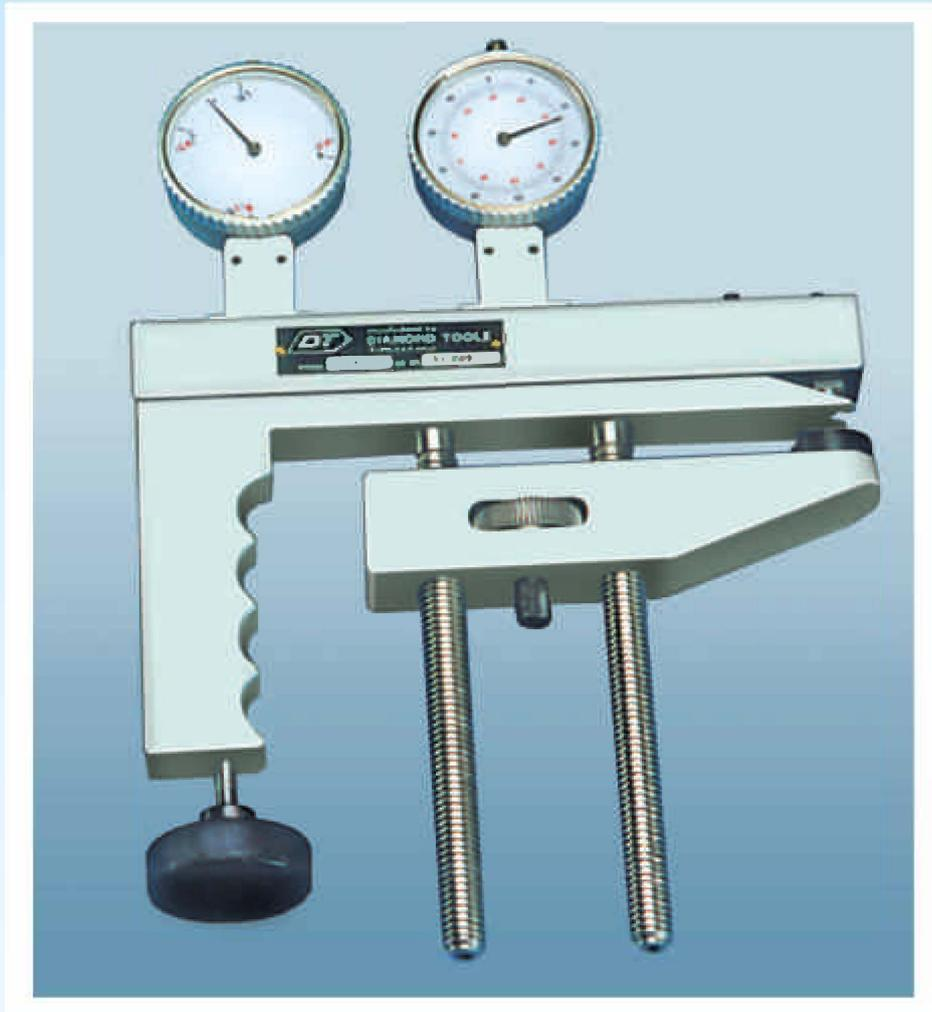
DT Portable Hardness Tester is developed to meet the demands of a light weight instrument which can be used to carry out tests by a universally recognised method of Hardness testing.
