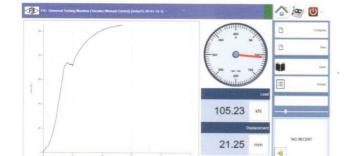
Real time values of load and displacement / extension used for plotting its graph & can be seen real time during testing & facility to convert the units simultaneously.
