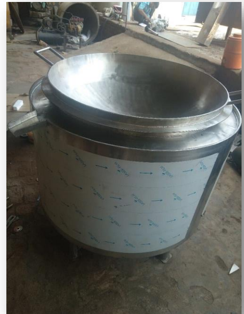
GAS AND DIESEL FURNACE(BHATTI)
