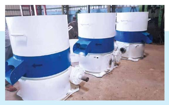
Palletiser (For Rice Bran) To make the pallets from conditioned bran. Capacity: From 50 Tons upto 150 Tons.
