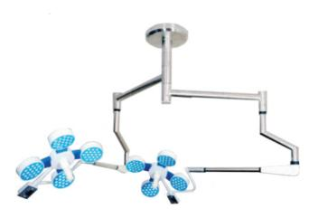
1,25,000 Lux Intensity · Intensity Satellite 1,25,000 Lux 100 - 150 mm **Spot Diameter** Depth Illumination 10 - 15 cm Colour Temp. 4000 - 4850 K Colour Rendering Index: 91 Ra Focusing Manual LED Average Life : >50000 Hrs Number of LED : 76 X 2 Diameter of Light 580mm X 2 Intensity Control : 10~100 Digital Power Supply : 220V/50Hz AC Power Consumption 40 X 2 Watt
