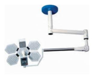
Luminance 1,75,000 Lux · Spot Diameter 100 - 180 mm Depth Illumination 15 - 21 cm Colour Temp 3200-5200 K Colour Rendering Index: 91 Ra Focusing Manual LED Average Life : >50000 Hrs Number of LED 178 Diameter of Light 693 mm : 10~100 Digital Intensity Control Power Supply 220V/50Hz AC Power Consumption AC, 55 Watts Special Function Memory
