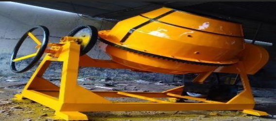
Heavy Duty Drum Type Concrete mixer 1 bag capacity Powered by 3 HP Motor
