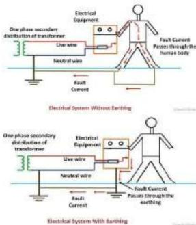
Earthing can be done by electrically connecting the respective parts in the installation to some system of electrical conductors or electrodes placed near the soil or below the ground level. The earthing mat or electrode under the ground level have flat iron riser through which all the non-current-carrying metallic parts of the equipment are connected.
