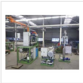
Steel Vapour Phase Drying Plant
