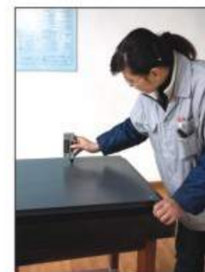
Coating Thickness Test 涂层厚度测试
