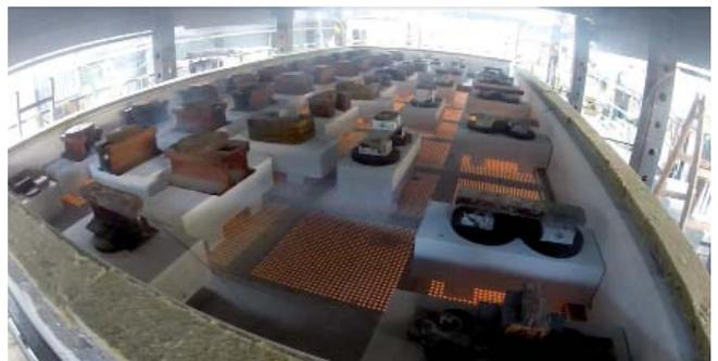
Lindner NORTEC is suited for the use in these areas due to its reaction to fire performance A1 according to EN 13501-1. The system has the respective F 30-AB / REI 30 classifications according to DIN 4102-4 respectively EN 13501-2.
