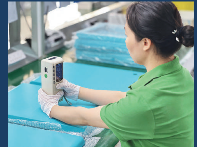
Color extractor detects the paint color difference of sheet metal
