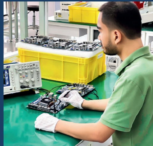
Oscilloscope detects PCB signal
