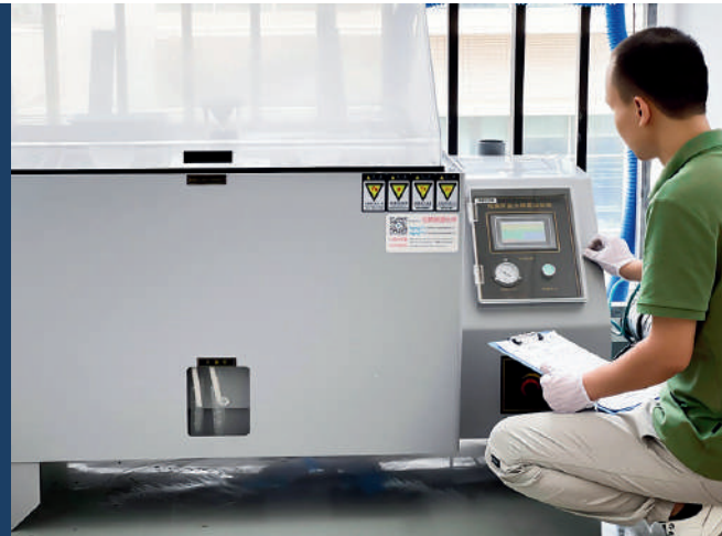
Salt spray tester tests the corrosion resistance of sheet metal
