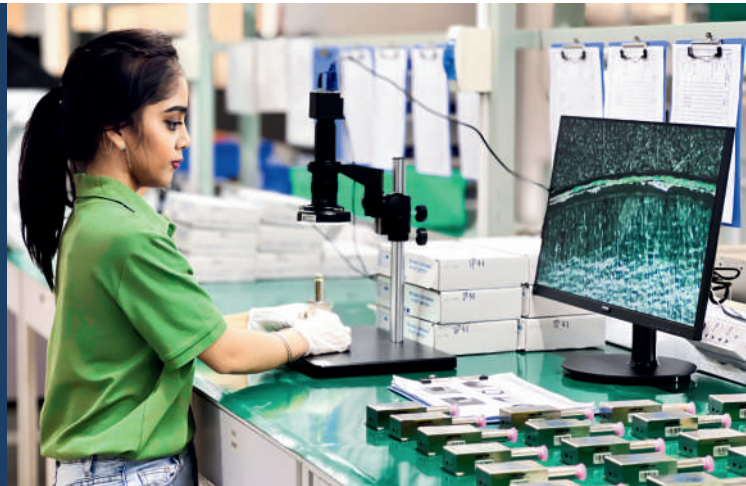
High-power microscope detects beryllium window quality of detector
