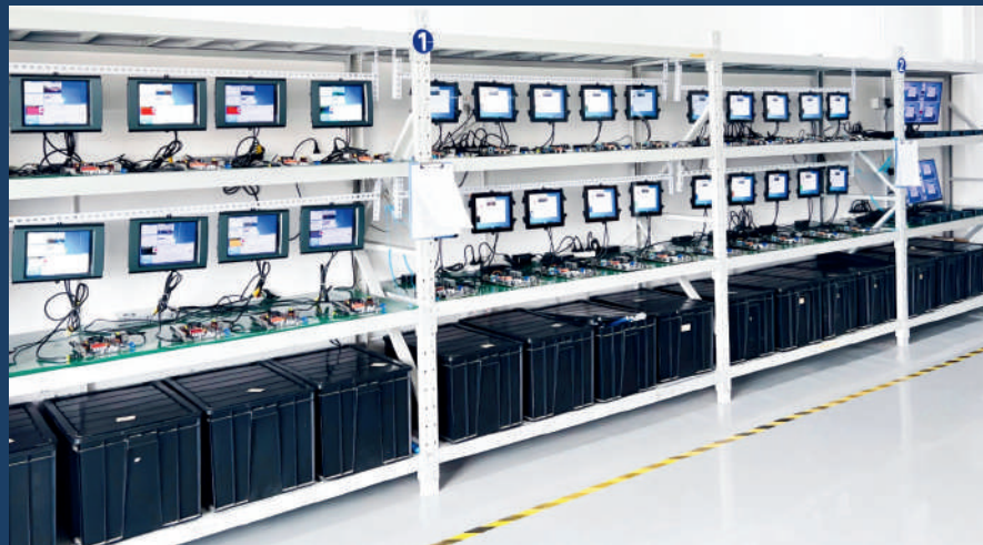
Aging testing for verifying the quality of PCB
