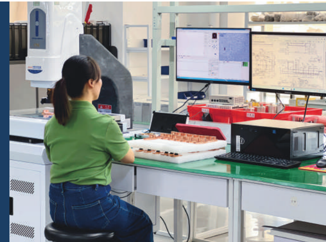
2.5-dimension measuring equipment measure the quality of collimator
