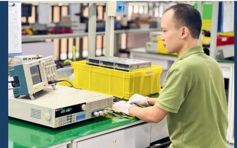
Power consumption and ripple detection of switching power supply
