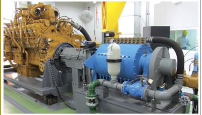
Our is fully equipped to complete your engine rebuild package by providing a comprehensive in-house engine testing facility using our recently commissioned dynamometers. These state of the art units allows us to test up to 4500HP and will ensure you are provided with accurate and certified fuel-burn emissions and power figures to achieve the best performance and fuel consumption from your engine right throughout its service life. A detailed report is provided with every engine tested.
