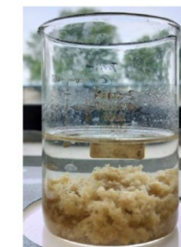
Coagulated supernatant and sludge separated by decanting into a beaker
